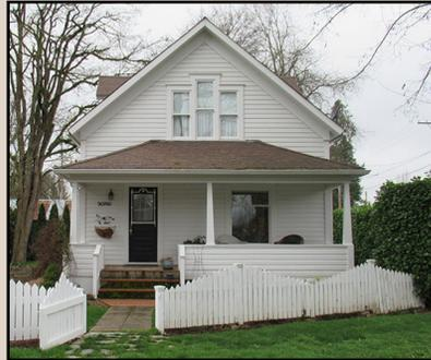
This is a one-and-a-half story, wood-framed rectangle structure with gable roof and corbeled brick center chimney. Shiplap siding and one-over-one, double-hung windows with molded hoods can be seen from the exterior. The porch has a hipped roof with tapered boxed columns and solid railing. It also has Italian elements such as Palladian windows on the second floor and narrow square bay to side street.
