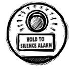
Do remember you can silence the audible alarm (it sounds like a smoke alarm) by pushing the lighted button directly above the "Push to Silence" label on the front of the electrical control panel until the alarm goes off. With normal use, the tank has a reserve storage capacity good for about 24 hours.
